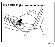
The Vehicle Identification Number (VIN) may be found in the location shown in the above illustrations. This number is used to register the vehicle. It is also used to assist your SUZUKI dealer when ordering parts or referring to special service information.
